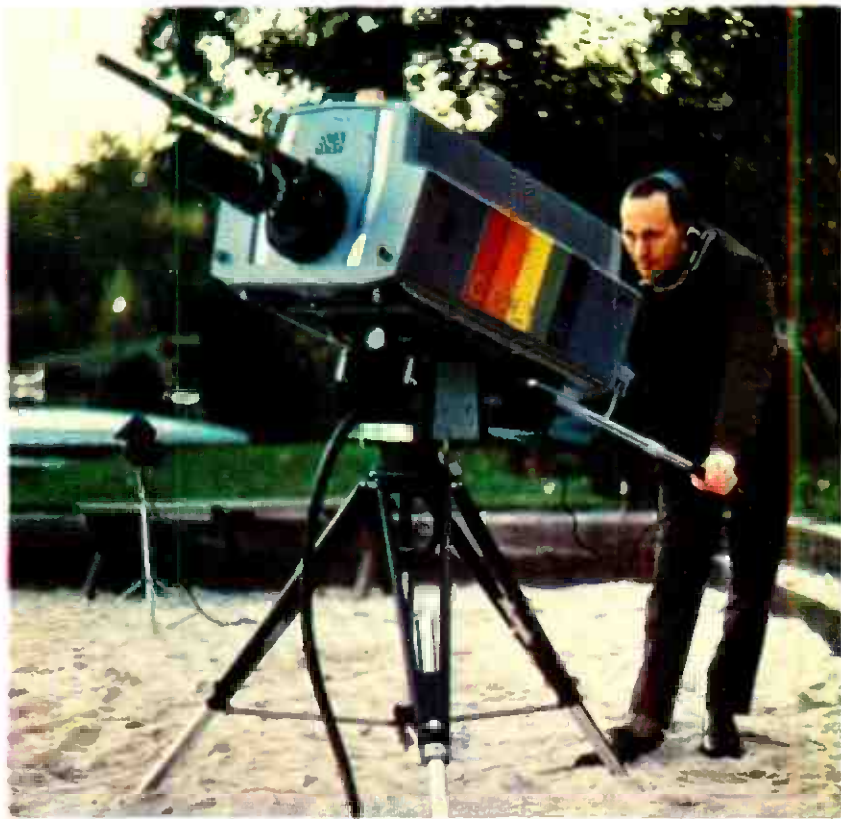
RCA Color Camera set up to test technical capabilities. A Casagrain type telescope, focal length 125 inches, was installed on the camera to produce the moon-shot shown here.
