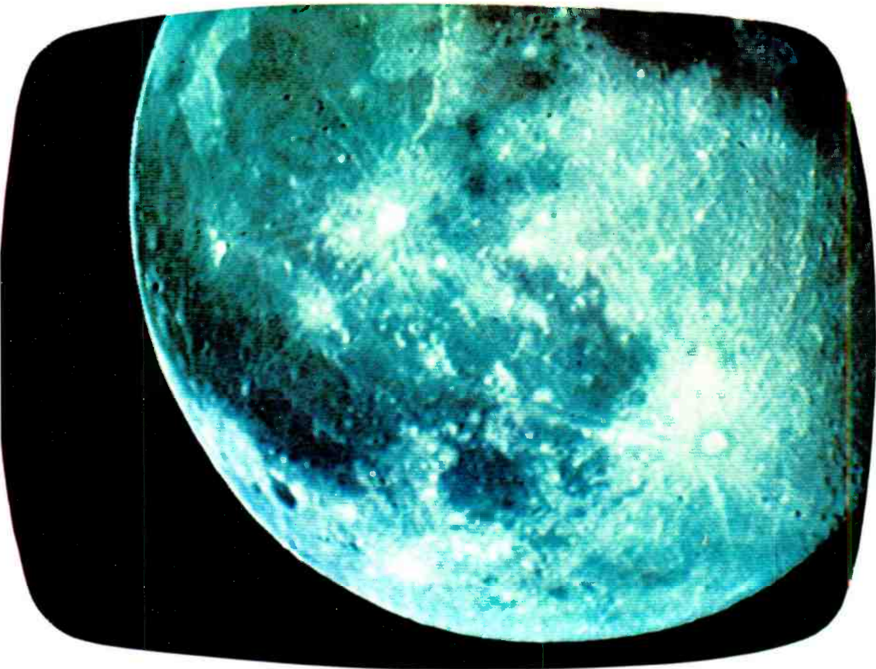
Unretouched photograph taken directly from monitor on Ektachrome daylight film, ASA 160, 2 1/4 x 2 1/4" format. Color temperature of monitor 9000K; color temperature of film 5500K.
